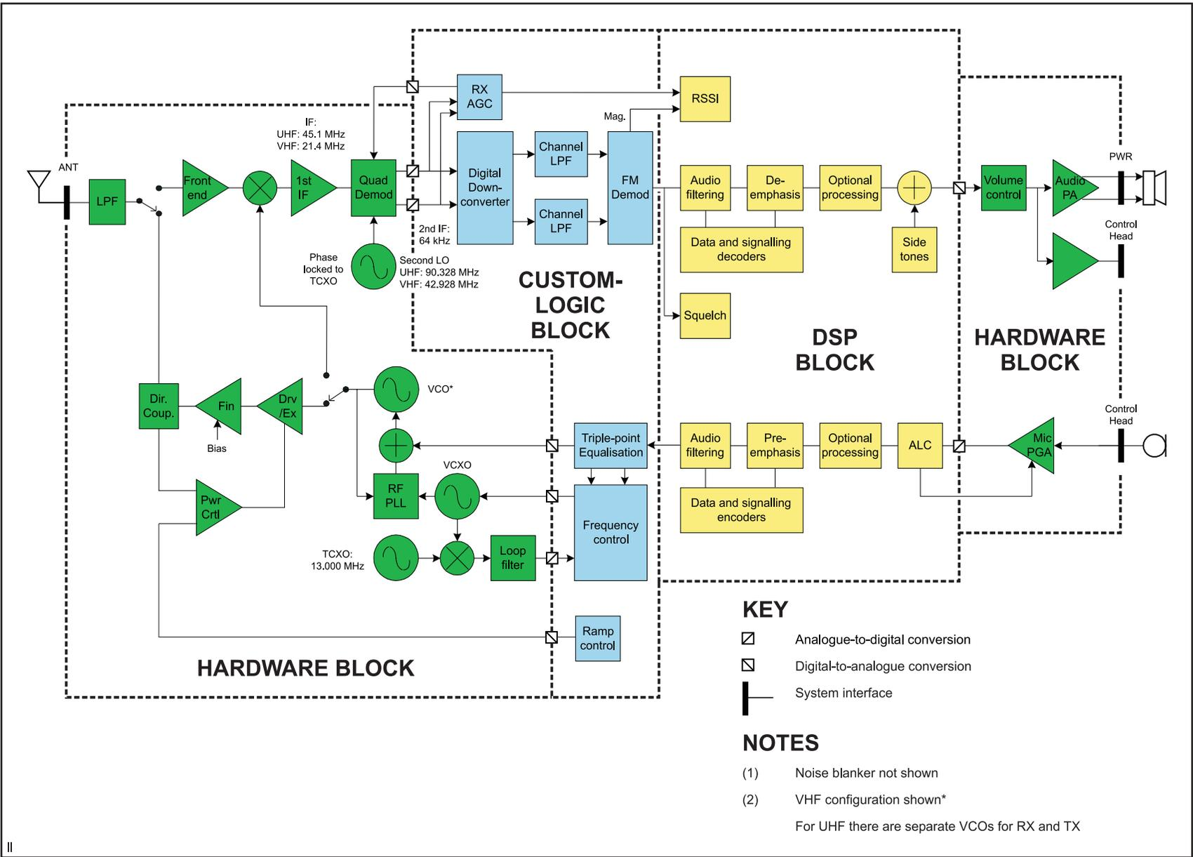
Figure 2.2 Architecture of the TM8100 transceiver
