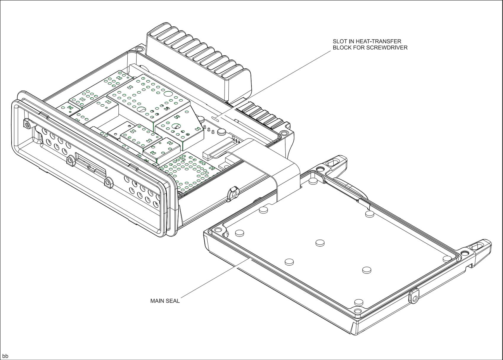
**Figure 3.7** Illustration of the lid removed from the chassis of the radio body, with an options board installed in the lid
